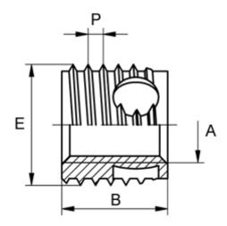
Female thread A = M16 Length B = 14 Male thread E = 20.0 Min hole depth blind hole = 17 Thread pitch P = 2.00
